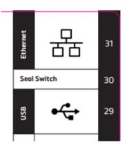
The seal switch is provided to protect only the front panel menu system. This protection mechanism prevents any inadvertent attempts to set any of the calibration parameters via the front panel menu system.
